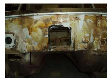
Original positioning of sound deadener under the window wipers. Firewall showing haphazard placement of yellow glue and luckily no signs of rust.
