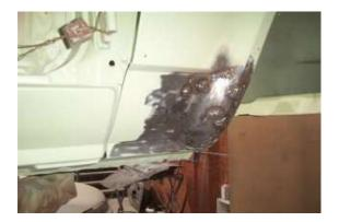
Rust holes in the lower guards were drilled out and butt welded and then hand filed and sanded.
