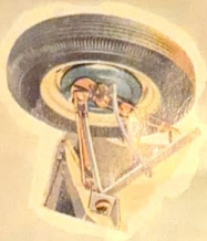
Independent torsion-bar front suspension absorbs every bump.
