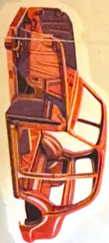
B.M.C. "Monocoque" type body is the same as the "Major's" shell... has enormous impact resistance, immense strength and minimum weight.
